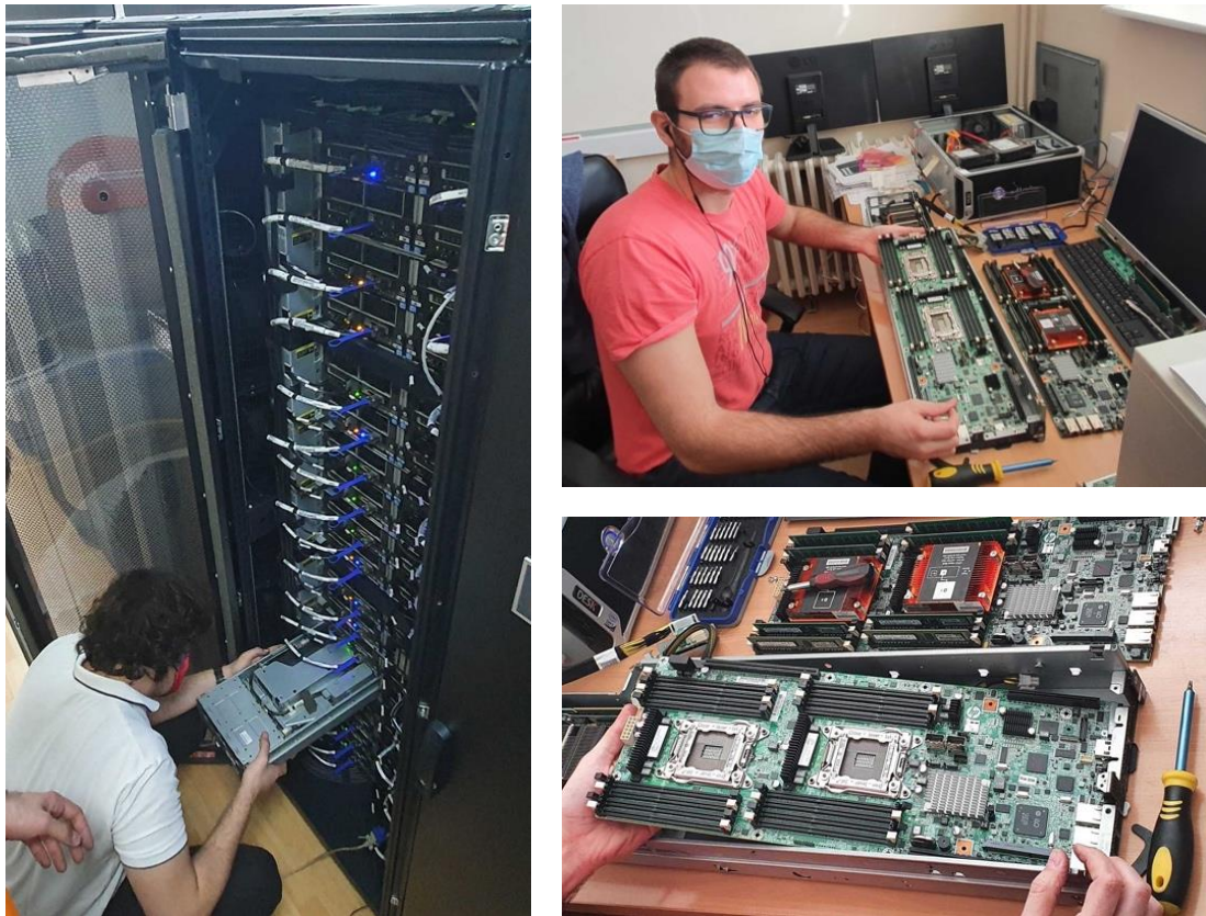
Figure 1: The Dialog and IPB teams in action during the motherboard replacement process.
